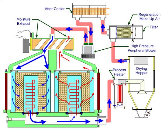
Figure 16: Low Heat Model (120°F to 250°F) Air Flow
